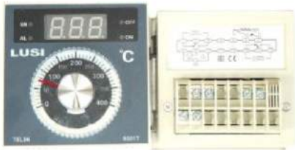
BAKING OVEN - TEMPERATURE CONTROLLER
